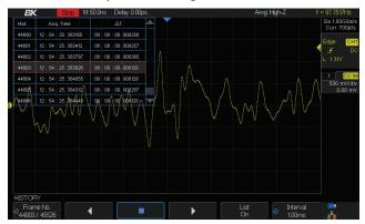
Quickly scroll through millions of points with History Mode's playback functionality to find difficult to capture events. Eliminate unnecessary idle signals and dead-time by selectivity capturing up to 80,000 segments.
