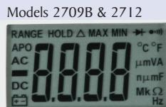
Large easy-to-read LCD with green LED backlight
