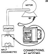
AC Motors & Generators: To carry out a basic insulation test on an ac motor or generator, connect the black alligator test lead to the frame or housing and contact the red high voltage probe to one of the motor terminals, or
