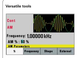
The 4045B provides AM and FM modulation along with linear/logarithmic sweep and built-in counter capabilities. Internal and external sources can be used for triggering and modulating the signal.
