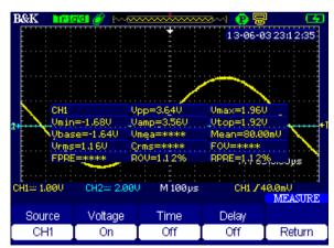
Figure 49 - All Voltage Measurements Display
