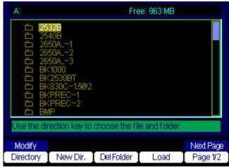
Follow the same instructions from section "3.7 Save/Recall Function" to create a directory and/or a new file, then select **Load** from the menu to save all recorded data into a new file on the external USB flash drive.
