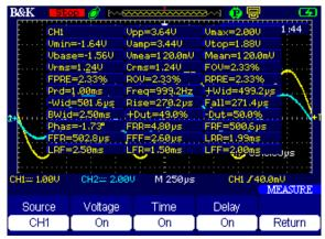
Figure 52 - All Measurements Display
