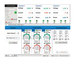
PC software is provided for front panel emulation, generating and executing test sequences or logging measurement data without the need to write source code.
