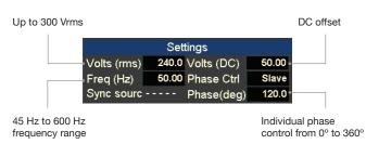
Set voltage, frequency, and phase directly from the front panel on each AC source.
