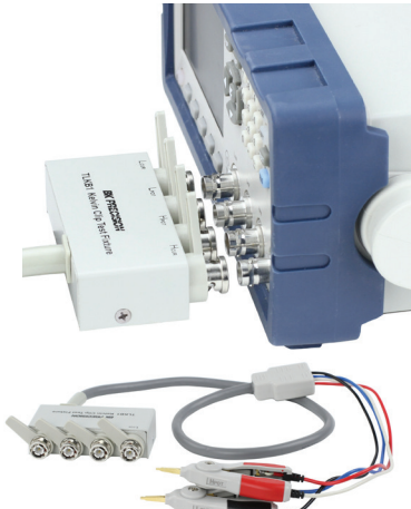
Kelvin clip test fixture
