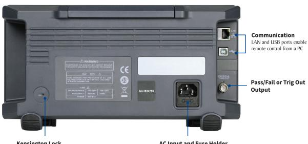
**Kensington Lock** Helps secure oscilloscope and prevent theft
