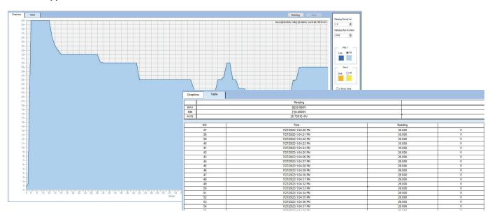
PC software is available for logging measurement data at specified intervals with date and time stamp. Log up to 100,000 data points in graph or table format. Measurement data recorded in the field can be imported using the software for analysis.
