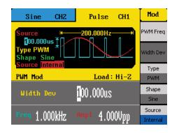
These instruments are capable of many different types of modulation for various applications. Modulate your waveforms with AM, DSB-AM, FM, PM, ASK, FSK, and PWM modulation schemes.
