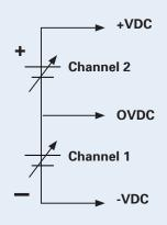
This feature is useful for powering bipolar circuits and devices.
