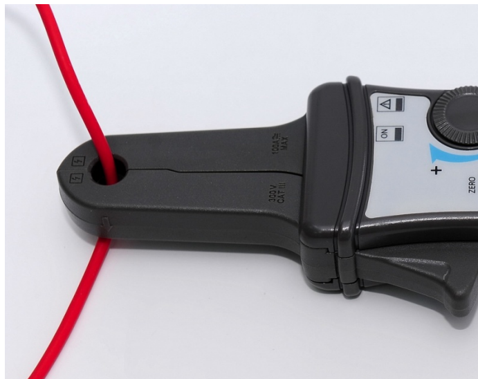
Figure 5: Connecting the CP62 current probe.
