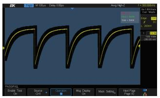
Perform up to 40,000 pass/fail decisions a second. Easy to generate masking templates help capture anomalies even with complicated waveforms.
