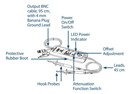
Figure 1 Front Panel Diagram
