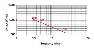
Figure 2 Derating Curve
