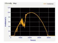
The PVS power supply outputs points on the I-V curve in 1 ms intervals to test the inverter's MPPT efficiency.
