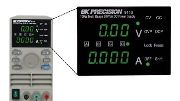
The 9110 is a new type of power supply. Unlike conventional power supplies with fixed output ratings, the 9110 automatically recalculates voltage/current limits for each setting. The 9110 provides 100 W output power in any Volt/Amp combination within the rated voltage (60 V) and current (5 A) limits. By providing greatly expanded choices of maximum power Volt/Amp combinations, users can cut down on the number of power supplies required and free up valuable bench space.
