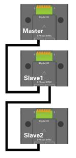
The TL983P adapters connect to the Digital I/O connector on the rear of the AC source. Standard RJ45 communication cables connect each adapter to route the 3-phase synchronization signal from the master to the slave units.
