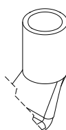
COLLETTO CHIUSO DA TUBO PIEGATO A 45° O 90° BARREL CLOSED BY A TUBE BENT AT 90° OR 45
