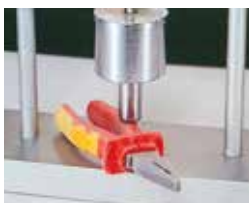
Prova alle basse temperature. Low temperature test.
