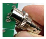
V-Bite<sup>®</sup> Edge-Mount connectors are fast and simple to install. Simply place the connector at a 45-degree angle to the PCB. Insert the PCB into the notched opening and push down onto the connector to seat it firmly in place.
