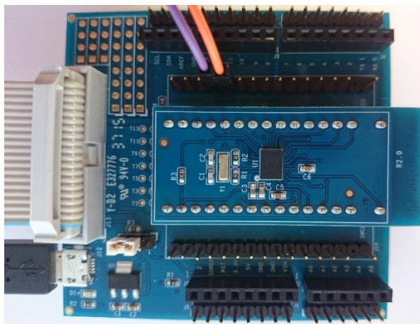
Figure 6 - Necessary connections to run reference examples
