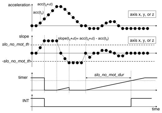
Figure 18: Signal timings no motion interrupt
