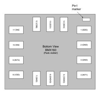
Figure 31: Pin-out bottom view
