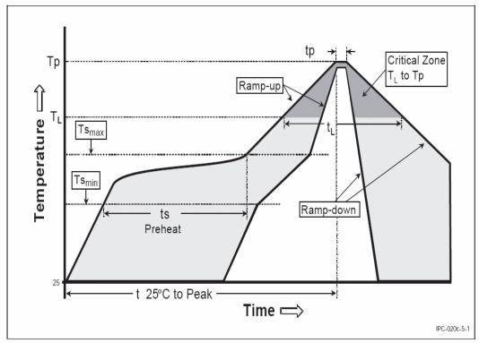
Figure 39: Soldering profile
