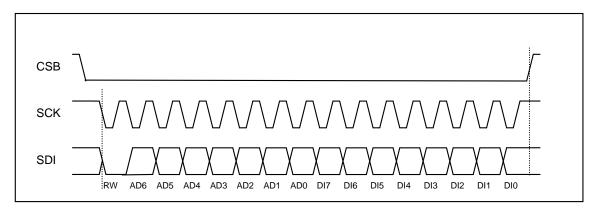
Figure 26: 3-wire basic SPI read or write sequence (mode "11")
