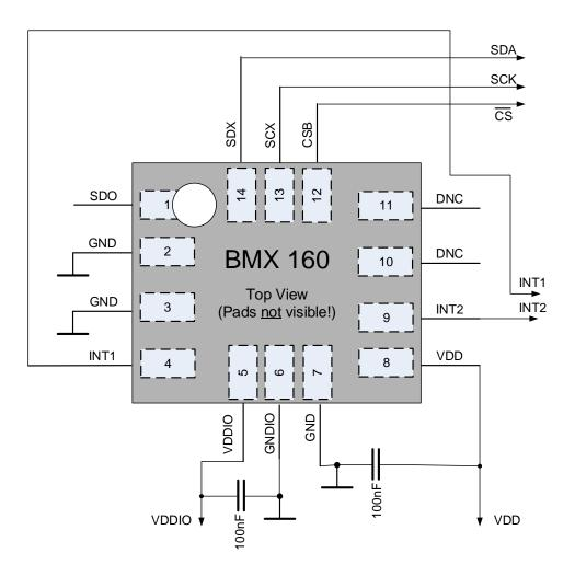
Figure 33: Only SPI 3-wire
