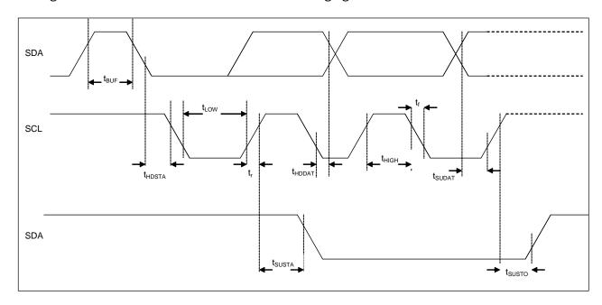
Figure 27: I2C timing diagram
