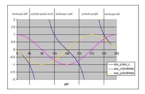
Figure 10: Angle-to-Orientation Mapping
