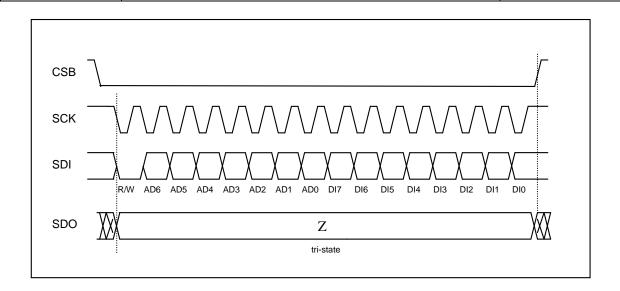
Figure 23: 4-wire basic SPI write sequence (mode "11")
