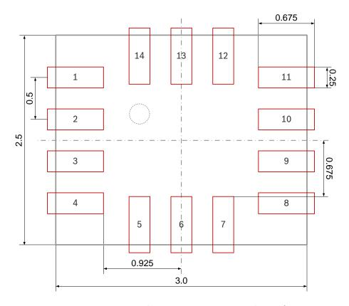
Figure 38: Landing pattern recommendation for BMX160
