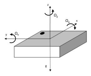
Figure 36: Definition of sensing axes orientation
