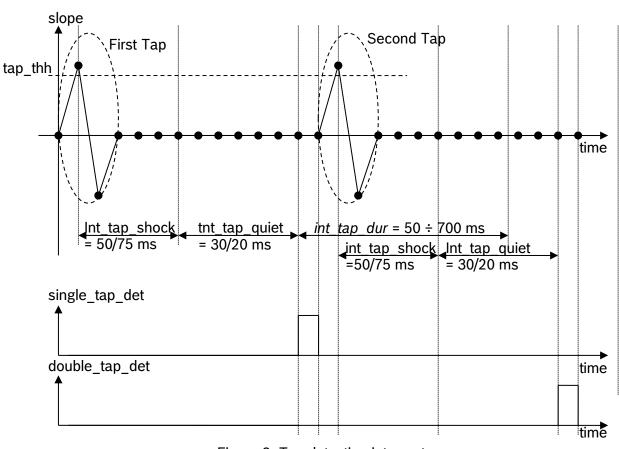
Figure 8: Tap detection interrupt
