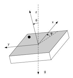
Figure 9: Definition of coordinate system with respect to pin 1 marker
