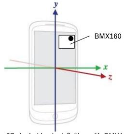
Figure 37: Android axis definition with BMX160
