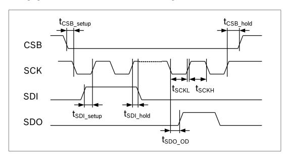
Figure 22: SPI timing diagram
