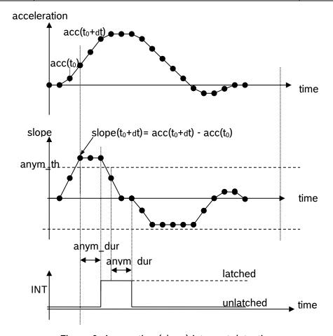
Figure 6: Any-motion (slope) interrupt detection
