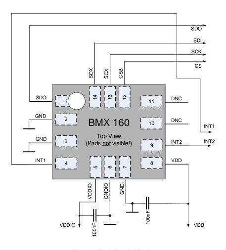
Figure 34: Only SPI 4-wire
