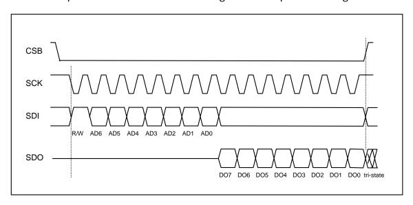
Figure 24: 4-wire basic SPI read sequence (mode "11")
