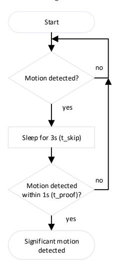
Figure 7: Block diagram of significant motion interrupt algorithm
