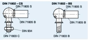
DIN 71802 - CS with screw stud, hex nut and circlip
