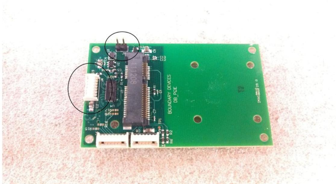
SABRE Lite/BD-SL-i.MX6. The cable must be plugged in with the orientation below, and requires a jumper to be installed.
