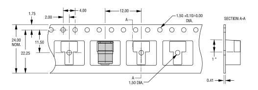
TOLERANCES: ±0.13 UNLESS OTHERWISE SPECIFIED DIMENSIONS: MILLIMETERS
