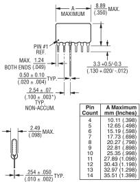
Maximum package length is equal to 2.54mm (.100") times the number of pins, less .005mm (.002")
