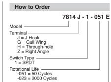
Optional Embossed Tape Designator (For pin styles J, G, Z only - omit for tube packaging)
