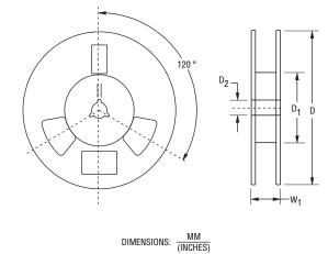
Devices are packed in accordance with EIA standard RS-481-A and specifications shown here.
