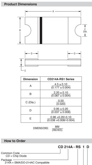
Model RS = Glass Passivated Fast Response Rectifier Series Maximum Average Forward Rectified Current
