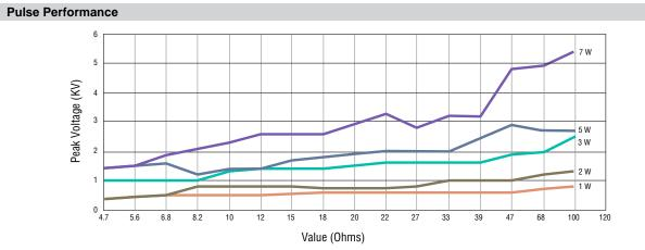
1.2/50  $\mu s$  Peak Voltage Limit (10 pulses at 10 sec. intervals,  $\Delta R$  < 5 %) NOTE: The voltage shown in these curves is the voltage across the resistor. The generator voltage will be higher due to the generator's internal impedance.
