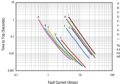
A - MF-USHT010KX B - MF-USHT016KX C - MF-USHT020KX D - MF-USHT035KX E - MF-USHT050KX F - MF-USHT050KX G - MF-USHT110KX H - MF-USHT125KX I - MF-USHT150KX
