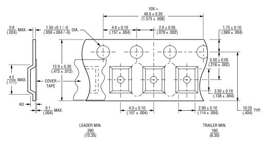
K0  $0.65 \pm 0.10$ MF-USML175/6 ~ MF-USML260/6, MF-USML175/12 ~ MF-USML260/12  $\overline{(.026 \pm .004)}$  $MF\text{-}USML300/6 \sim MF\text{-}USML700/6, MF\text{-}USML300/12 \sim MF\text{-}USML550/12$
