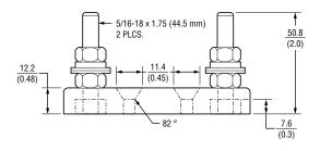
TOLERANCES HOLE DIAMETERS: ±0.381 (± 0.015)
