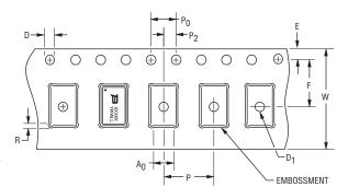
The type of corner on carrier will vary at different assembly sites.
