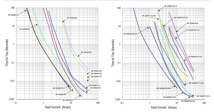
The Time to Trip curves represent typical performance of a device in a simulated application environment. Actual performance in specific customer applications may differ from these values due to the influence of other variables.
