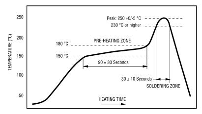
PEAK: 250 +0/-5 °C, 5 seconds PRE-HEATING ZONE: 150 to 180 °C, 90  $\pm$  30 seconds SOLDERING ZONE: 230 °C or higher, 30  $\pm$  10 seconds
