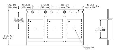
DIMENSIONS:  $\frac{\text{MM}}{\text{(INCHES)}}$  USER DIRECTION OF FEED QUANTITY: 800 PCS. PER REEL
