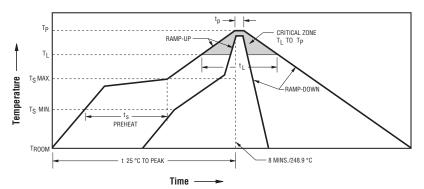
Ramp-up rate = 3 °C/sec. max. Ramp-down rate = 6 °C/sec. max.  $T_L$  = 217 °C  $t_L$  = 60-150 sec.  $T_p$  = 250 °C ±3 °C
