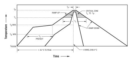
Ramp-up rate = 3 °C/sec. max. Ramp-down rate = 6 °C/sec. max.  $T_L = 217 °C t_L = 60-150 sec.$   $T_p = 250 °C \pm 3 °C$ Time within 5 °C of actual Peak Temp  $(t_p)2 = 20$ ~40 sec.  $T_S min = 150 °C T_S max = 200 °C$  $T_S min to T_S max = 60-180 sec., 25 °C to Peak Temperature = 8 min. max.$
