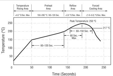
Peak Temperature: 250 ° C max. Max. Peak Temperature -5 °C: 30 sec. max. Time Above 217 °C: 60-150 sec. max.
