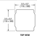
† Dimension does not include termination. For maximum overall dimensions with termination, add 0.1 mm (.004 in.).
