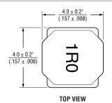
† Dimension does not include termination. For maximum overall dimensions with termination, add 0.1 mm (.004 in.).
