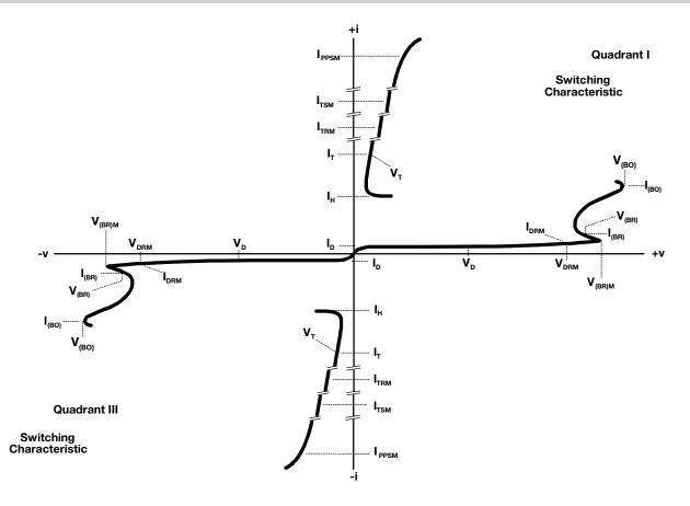
Figure 1. Voltage-Current Characteristic for the Ring and Tip Terminals All Measurements are Referenced to the Ring Terminal
