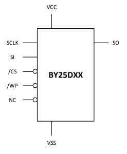
Figure 2. Pin Configuration SOP8 150/208 mil
