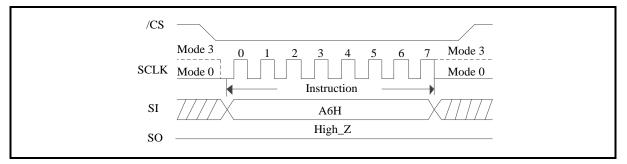
Figure 168. SPB Lock Bit Clear (QPI Mode)
