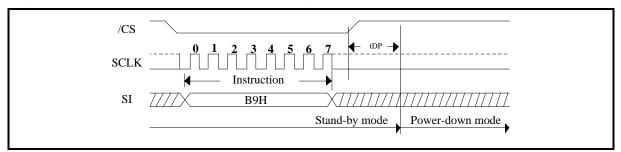
Figure 110. Deep Power-Down Sequence Diagram (SPI Mode)
