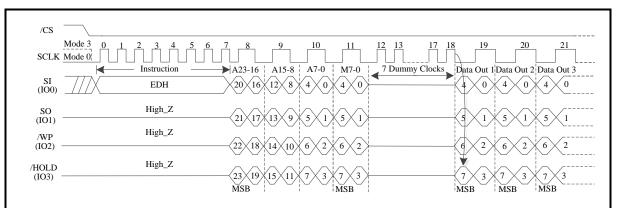
Figure 72. DTR Fast Read Quad I/O (SPI Mode/4-Byte Address Mode; Initial instruction or previous (M5-4 $\neq$ (1,0)))
