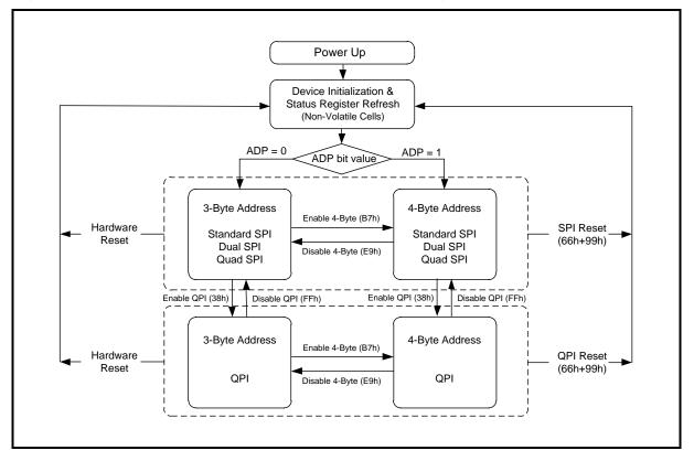
Figure 5. BY25Q256FS Serial Flash Memory Operation Diagram
