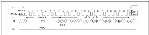
Figure 166. Write Lock Register (QPI Mode)
