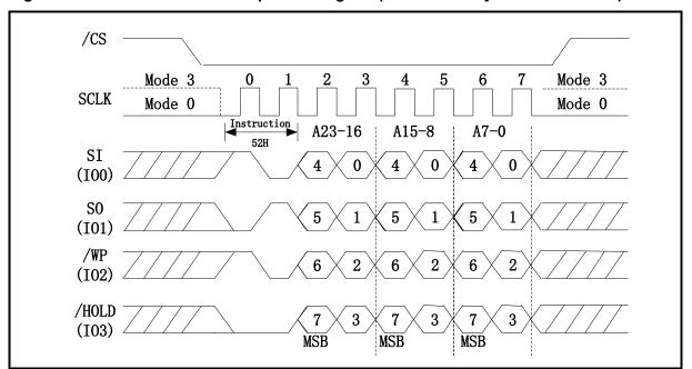
Figure 147. 32KB Block Erase Sequence Diagram (QPI Mode/3-Byte Address Mode)
