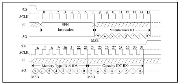
Figure 105. JEDEC ID Sequence Diagram (QPI Mode)
