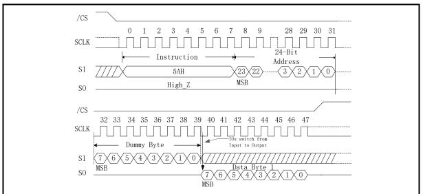
Figure 129. Read Serial Flash Discoverable Parameter instruction Sequence Diagram (QPI Mode)
