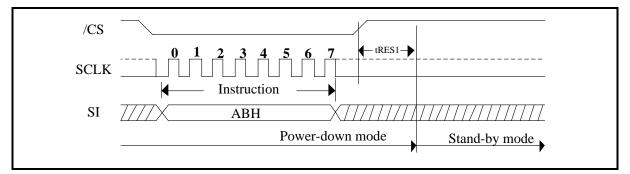
Figure 112. Release Power-Down Sequence Diagram (SPI Mode)
