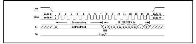
Figure 22. Write Status Register Sequence Diagram-01/31/11H 1byte (QPI Mode)
