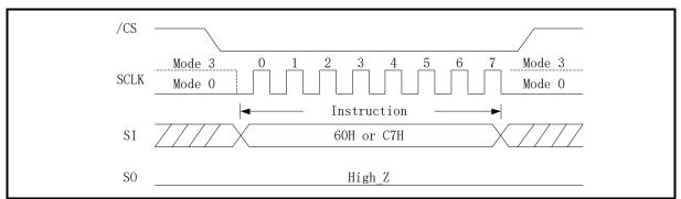
Figure 157. Chip Erase Sequence Diagram (SPI Mode)
