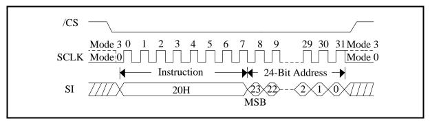
Figure 139. Sector Erase Sequence Diagram (SPI Mode/3-Byte Address Mode)
