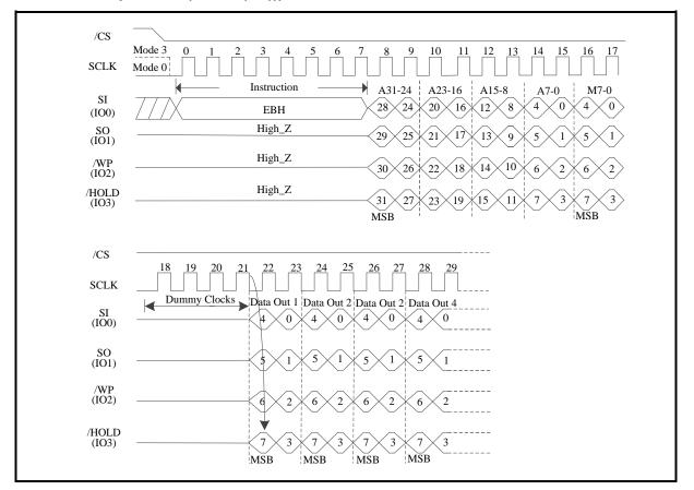
Figure 64. Quad I/O Fast Read Sequence Diagram (SPI Mode/4-Byte Address Mode; Initial instruction or previous (M5-4 $\neq$ (1,0)))
