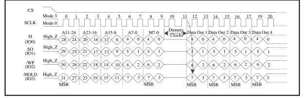
Quad I/O Word Fast Read with "8/16/32/64-Byte Wrap Around" in standard SPI mode
