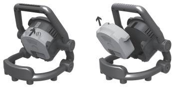
The battery can be easily and quickly replaced. Press the lock (F) forward and then slide the battery up and out, see drawing. It is therefore possible to charge one battery and continue working with a separately available replacement battery.
