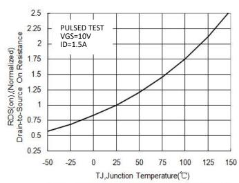
Figure 8.On-Resistance Variation with Temperature
