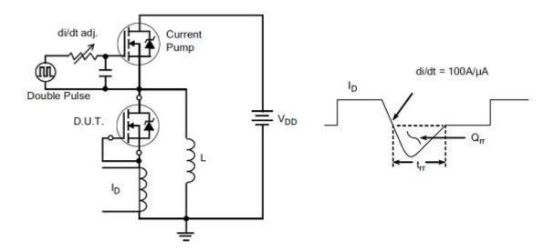
Diode Reverse Recovery Test Circuit
