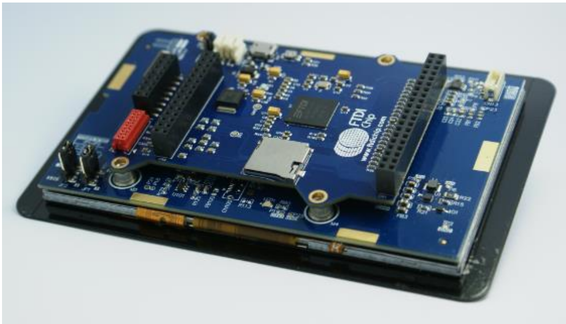
Figure 7-1 – ME813A-WH50C connects to MM900EV1A Module
