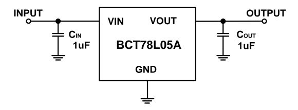
NOTE: If has a large Load Transient in the application, recommend using 4.7uF or more in Cout.
