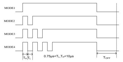
**Figure 14 One Wire Pulse Control**
