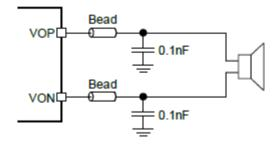
Figure 17 Ferrite Chip Bead and capacitor
